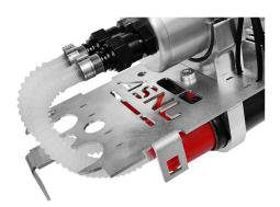
The "BBS" comes with a bespoke stainless steel module lid and with up-rated scavenge fittings for improved module filling. The filter unit is a unique twin inlet design for high flow. We supply a 6 micron filter pre-fitted and an additional spare. The hose supplied is an OEM spec type, compatible with all fuels and rated to IO bar.
