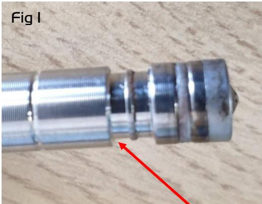
Bosch type injector with edge to retain the Graphite seal.
