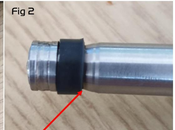
Denso type injector with no edge to retain the Graphite seal.
