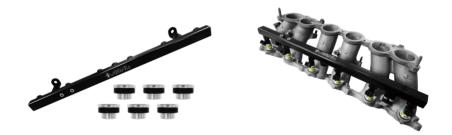
Our Toyota 2JZ VVTI rail is designed to convert the old side feed set-up found in the VVTI engine to top feed. This fitment can support our ASNU injectors from 300cc up to ISOOcc in our standard fitments. The kit comprises of I x rail, 2 x fitting bolts and 6 x manifold adapters.
