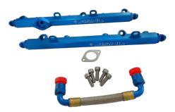
The ASNU R35 GTR fuel rails are designed for high performance engines, as our rails have a 17mm internal bore; far larger than the 3/8" OEM fuel rails, allowing a much higher flow of fuel. Our rails allow the retention of the stock rail mounted fuel damper using our spacer plate and are supplied with -8AN Orb fittings at each end.
