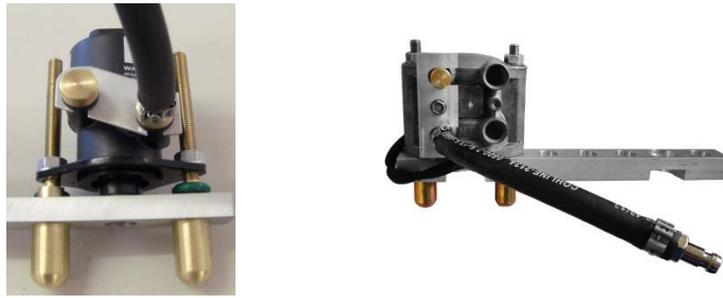
6.) Fit fuel connections for the injector type and connect to the ASNU machine
