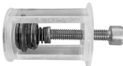
The solenoid pack and filter can be cleaned mounted upside down in the specific cleaning tray 185T supplied with the kit. The filter element mounted around the middle of the injector should be completely immersed in cleaning fluid. The mesh filter screen on the solenoid pack is washed clean in situ during the cleaning cycle. The cleaning of the solenoid pack must be done in clean ultrasonic fluid.
