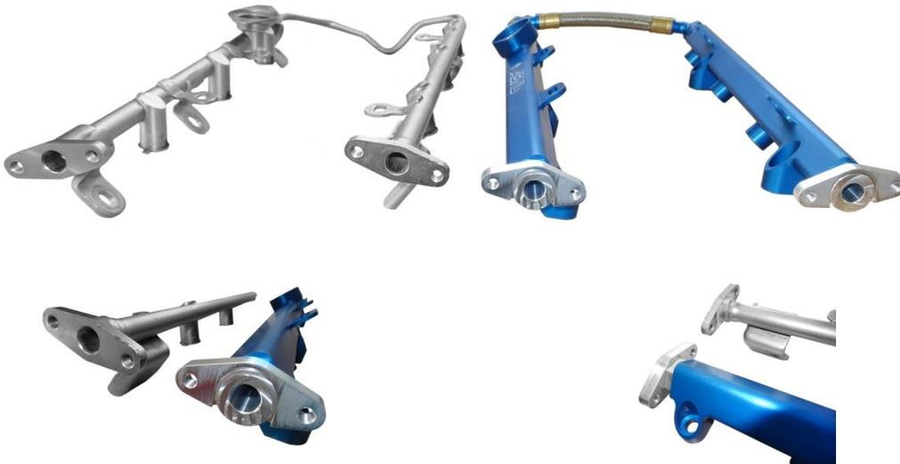
We can supply the correct fittings to go from 3/8th to -8 for the required hose connections if the OE under body fuel lines are to be retained (which we do not recommend for high HP applications).
