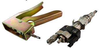
. Undo grub screw on the ASNU 84 Tool
