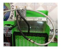
6.) Fit fuel connections for the injector type and connect to the ASNU machine
